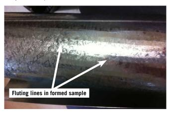
It is a naturally occurring characteristic of annealed low-carbon steel and is influenced by the steel chemistry, cold-reduction practices and annealing cycles. It is associated with material that has an upper and lower yield point, or yield point elongation (YPE) and may also be referred to as Luder Lines, stretcher strain, or discontinuous/non-uniform yielding.
